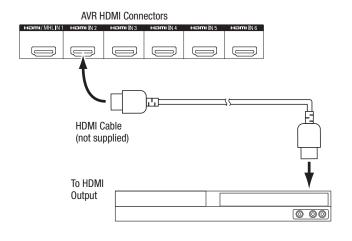
**HDMI-Equipped Source Device**
