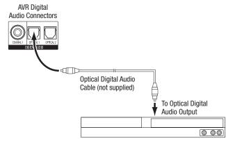
Optical-Equipped Source Device
