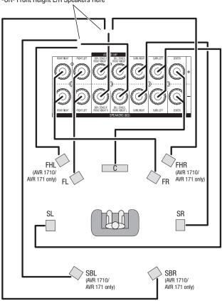
$\ensuremath{\text{NOTE:}}$  If you installed front height speakers, connect them as shown for the SBL and SBR speakers.
