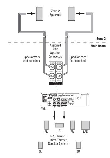
**B. Connect an external amplifier to the AVR's Zone 2 Out connectors.** This method offers the benefit of retaining a 7.1-channel home theater in the main room simultaneously with multizone operation, although it does require an additional amplifier for Zone 2.
